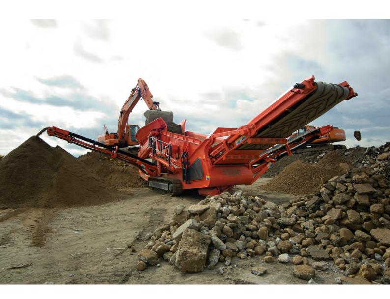
The Sandvik QE340 is a heavy duty, tracked, self-propelled, open flow screening and stockpiling system. This revolutionary machine has been purpose built for the recycling and quarrying markets. Based on in-depth customer and market analysis, the QE340 has been developed in order to deal with customer's real requirements, which traditional screening solutions are unable to adequately cater for.
