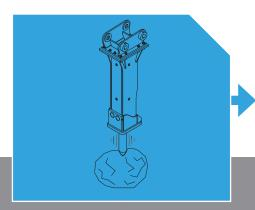
When the breaker operates in normal conditions the tool is in contact with the rock and strikes.
