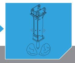
There is no resistance under the tool... all the energy remains trapped inside the breaker... as a famous scientist said: "nothing is lost, nothing is created, everything is transformed". An operator often continues to operate when the rock is broken... this is called "blank firing".
