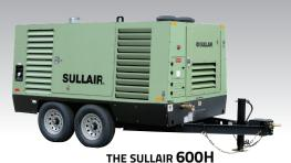
600 cfm at 150 psiq - 17 m<sup>3</sup>/min at 10 bar
