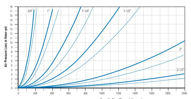
**Example #1**: A Customer has a 185 cfm air compressor equipped with 100' of 3/4" hose to operate a Sullair 90 pound paving breaker. The 90 pound paving breaker requires 62 cfm to operate. How much pressure loss can the Customer expect at the tool if the compressor is providing 100 psig inlet pressure?
