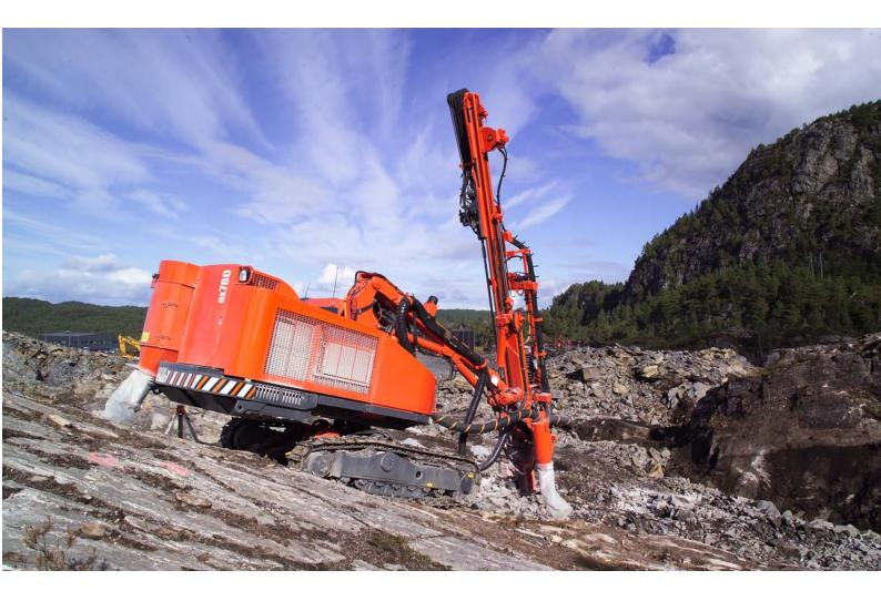
Sandvik DX780 is a hydraulic, self-propelled, self-contained, crawler based surface drilling rig equipped with a cabin (F.O.P.S. and R.O.P.S.) and rod handling system.
